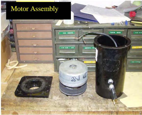
Figure 5-11 Blower Motor Maintenance
