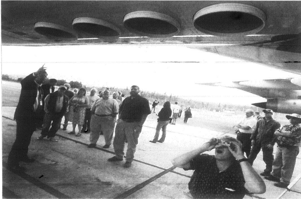
Eric Engman/ News-Miner Evergreen Aviation senior vice president Sam White, far left, talks about the four nozzles that dispense retardant as Evergreen Aviation shows off its 747 Supertanker firefighting aircraft Wednesday. Tom George of the Aircraft Owners and Pilots Association, bottom right, photographs the nozzles.
