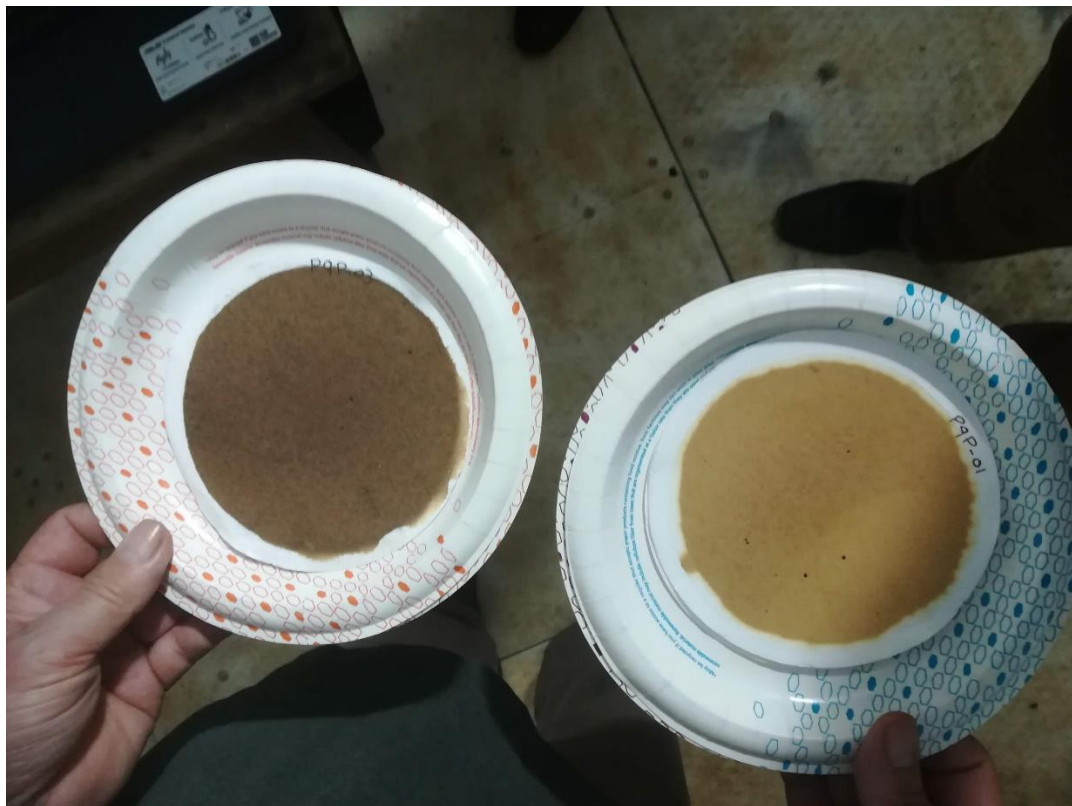
Pic. 4 Gravimetric measurements: left without OekoTube inside (0.5814 g), right with OekoTube inside. (0.2581 g)
