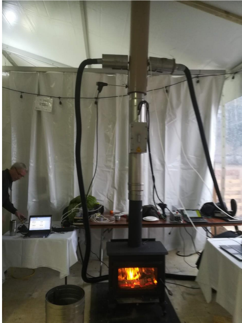
Pic.3 Testing of the Englander NC-13 using 2 Codars
