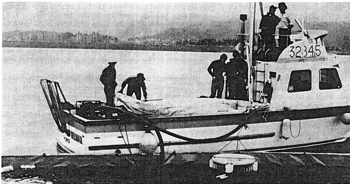
Oil spill cleanup equipment like this could be used in the event of a spill. The oil is contained by a floating boom and skimmed off the surface.
