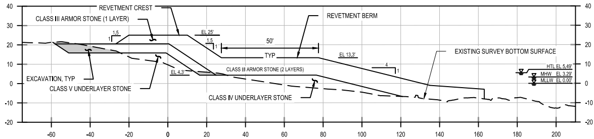
3 SECTION VIEW - SHORELINE REVETMENT SCALE: 1" = 50'
