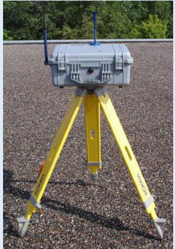
Stationary monitors are frequently used by rural communities to monitor dust. Photo from DustTrak manual.
