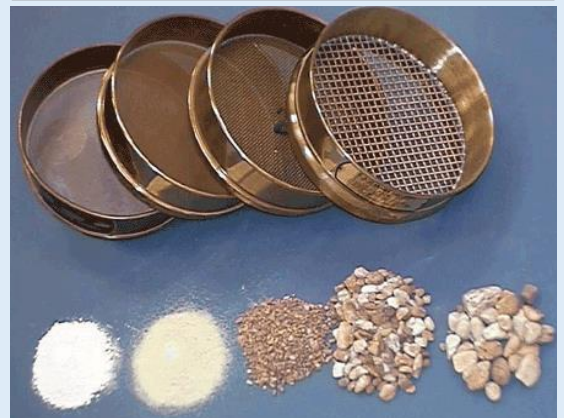
Sieved gravel showing various sizes of material. An aggregate gradation is mostly composed of gravel, sand, and silt. (Photo from ADOT&PF presentation, "Alaska Gravel Road Problems.") http://cem.uaf.edu/media/188432/gravel-roads-lecture_mchattie_june-2015.pdf
