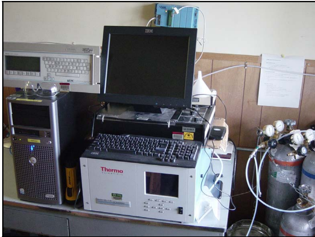
Figure 2-2 TECO 48 CO Analyzer with Data Acquisition System Garden Monitoring Station
