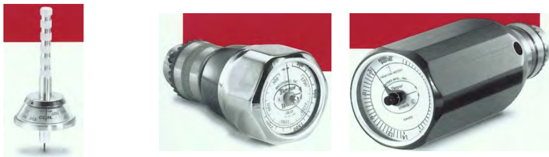
Figure 2-9 Waters Torque Watches: Low-Range 366, Medium Range 651, High Range 940. 19
