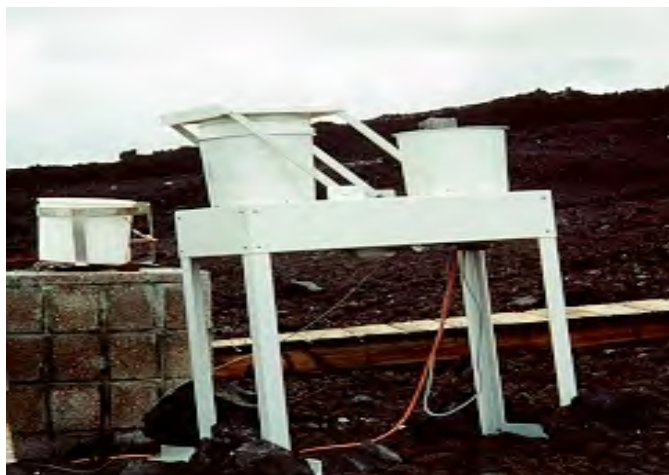
Figure 4.2 Automatic Wet/Dry Precipitation Collector
