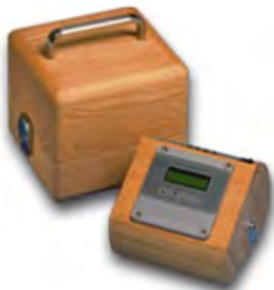
Figure 7.2 Portable Digital Barometer. Source:
