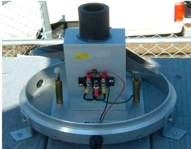
Figure 4.4 Tipping Bucket Without the Shield
