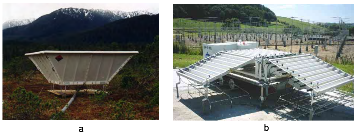
Figure 8.7 Photographs of Types of Radar Wind Profilers: (a) Phased-Array System and (b) Fixed-Axis Antenna System
