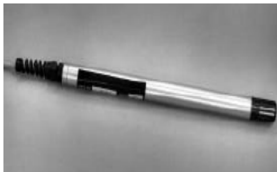
Figure 5.2 A Typical RH Probe. Source: < http://www.metone.com/ >
