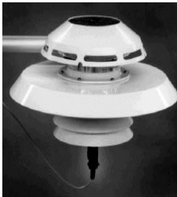
Figure 3.3 A Motor-Aspirated Shield. Source: < http://www.metone.com/ >
