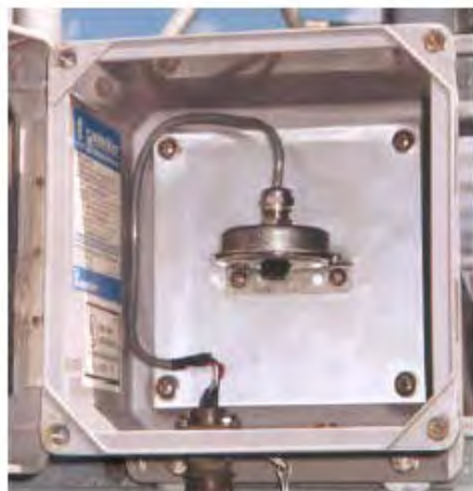
Figure 7.3 NEMA 4X Enclosure. Source: http://www.climatronics.com/pdf/products/sensors/102270.pdf
