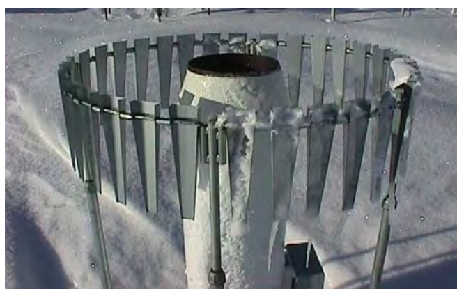
In below-freezing conditions when the catch in a gauge is snow or some other form of solid precipitation, the collector/funnel of non-recording gauges and the funnel in recording gauges must be removed. Some instruments are available with built-in heater elements that are thermostatically controlled. An effective heater for conditions that are not too severe is an incandescent lamp installed in the housing of the gauge. Caution should be exercised because too much heat will result in Figure 4.5 Example of an Alter Wind Shield
