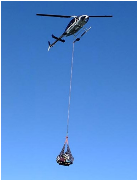
Figure 23. Helicopter Sling Load Operations
