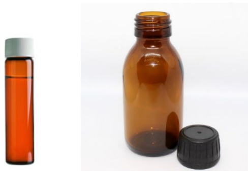
Figure 2. Example of 40 mL glass vial or 125 ml brown glass bottle for TOC sampling
