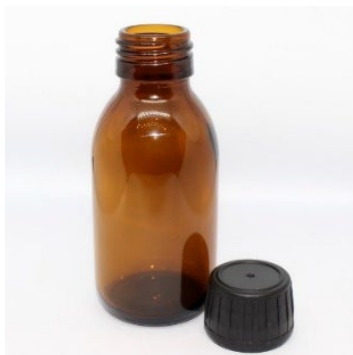
Figure 16. Example of 250 mL brown glass bottle for HAA5 sampling
