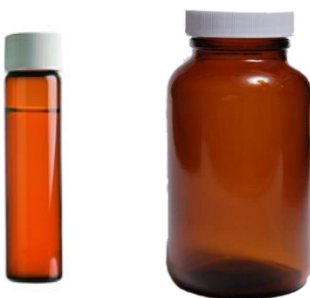
Figure 6. Example of 40 mL glass vial or brown glass bottle for SOC sampling
