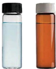
Figure 5. Example of 40 mL glass vials with Teflon septum cap for VOC sampling
