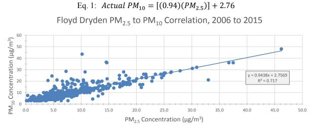
Figure 5-3: Correlation between PM<sub>2.5</sub> and PM<sub>10</sub> at Floyd Dryden from 2006-2015. Concentrations <3µg/m<sup>3</sup> were excluded.
