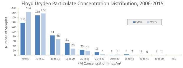
Figure 5-2: Distribution of Particulate Matter Concentrations over 2006 to 2015. Concentration pairs <3µg/m<sup>3</sup> were excluded.
