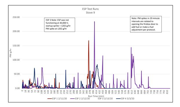
Figure 14. Non-Catalytic Stove 9 ESP Test Runs PM Rates
