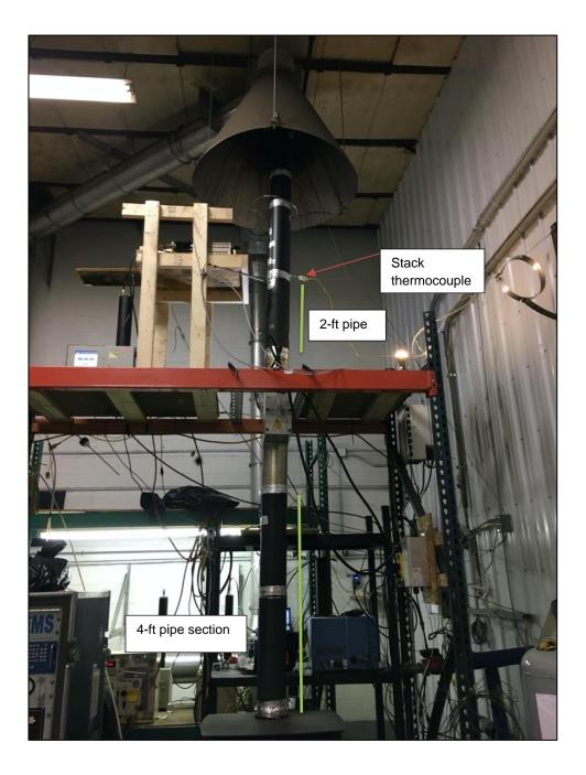
Figure 5. ESP installed on Cordwood Stove
