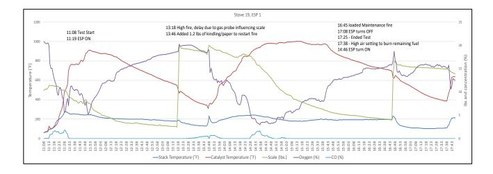
Figure 15. Catalytic Stove 19 ESP Test Run
