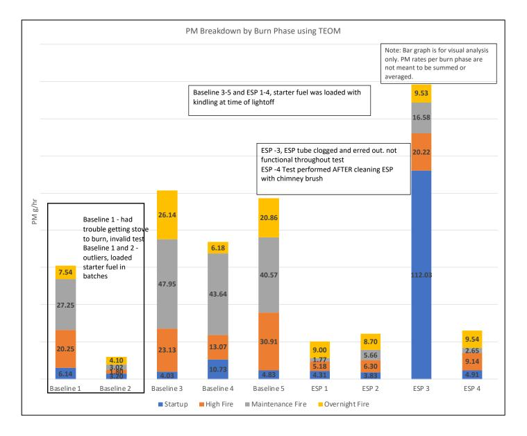
Figure 6. Non-Catalytic Stove 9 PM Phase Comparison
