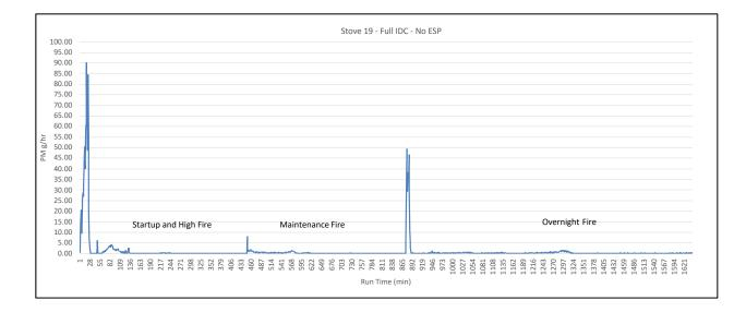
Figure 2. Catalytic Stove 19 IDC Test Example
