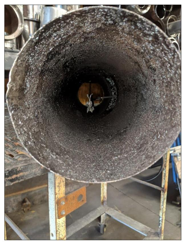
Figure 12. ESP After Cleaning
