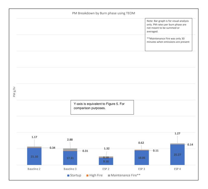
Figure 8. Catalytic Stove 19 PM Phase Comparison
