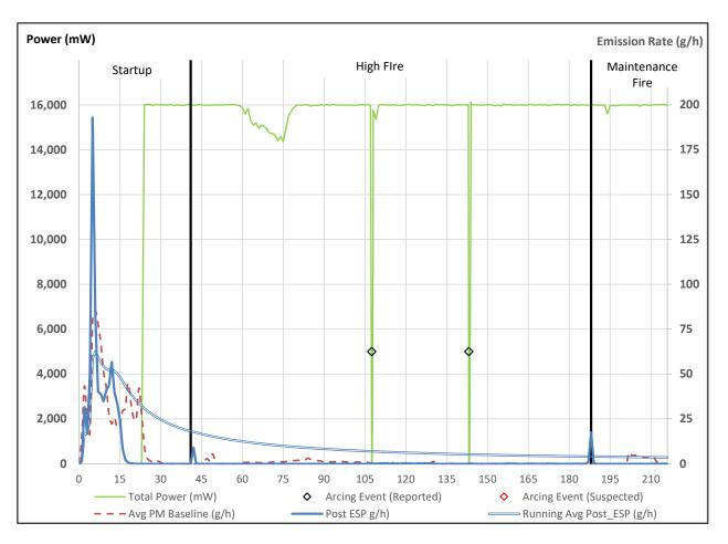
Figure 9 Catalytic Stove 19 with ESP, Run 3, Entire Run (minutes 0-216)
