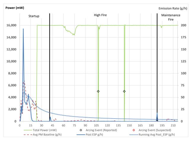
Figure ES-3 Catalytic Stove with ESP, Entire Run (minutes 0-216)
