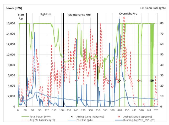
Figure ES-1. Non-Catalytic Stove 9 with ESP, Run 4, Entire Run (minutes 0-576)
