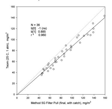
Dilution tunnel PM measured with the TEOM is highly correlated with the Method 5G filter pull PM, and is about 11% lower, with a zero intercept. Thus 5G filter pull equivalent data can be obtained from TEOM PM data by use of a simple linear correction of 11%. These results are consistent with the results of TEOM and filter pull PM from the BNL work shown in Section 2.2 above.
