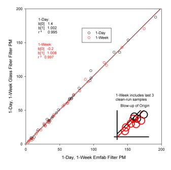
The 0-day equilibration glass fiber filter PM has a large positive bias on several samples that goes away after 1-day equilibration. Figure 2 shows very good correlation of the Teflon membrane filter samples with the Emfab samples at all equilibration times. This confirms it is the 0-day glass fiber PM samples that are unstable, not the Emfab 0-day samples. The 1400 Teom data also support this conclusion (see below).
