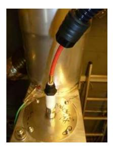
4. The high voltage cable must be fastened properly.
