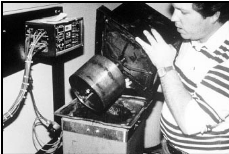
Darwin Wright at Photolab in Anchorage uses an electrolytic silver recovery system.
