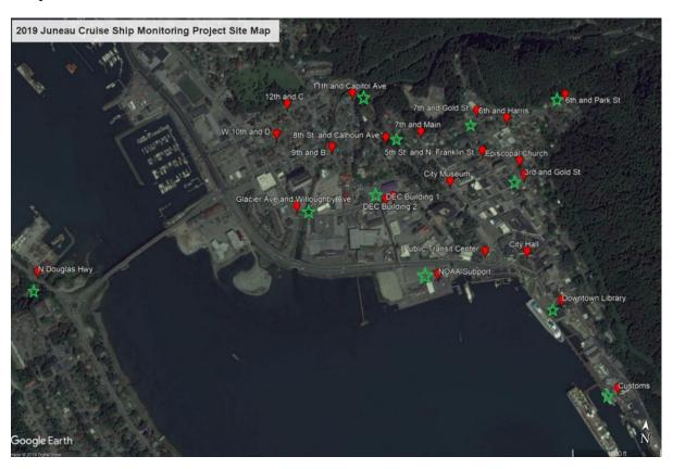
Figure ES-1. Cruise ship monitoring PurpleAir site locations. Red pins are PA site locations and green stars indicate sites used as SO2 sampling sites.
