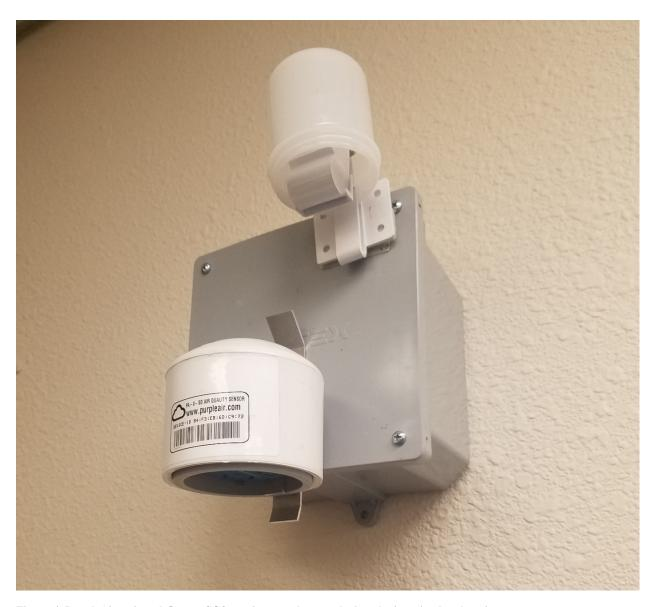
Figure 4. PurpleAir unit and Ogawa SO2 passive sampler attached to the junction box housing.
