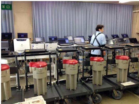
Figure 3. Banks of scintillators used to count radiation levels in produce, milk, and meat from Fukushima City. Testing is free for residents' food from private gardens.
