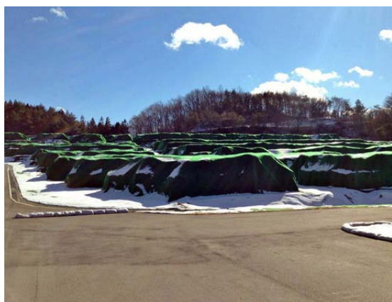
Figure 2. Temporary storage for radioactive waste from the decontamination of Kawauchi village. The waste is stored in impermeable bags that are stacked and covered to prevent sunlight from degrading the bags.
