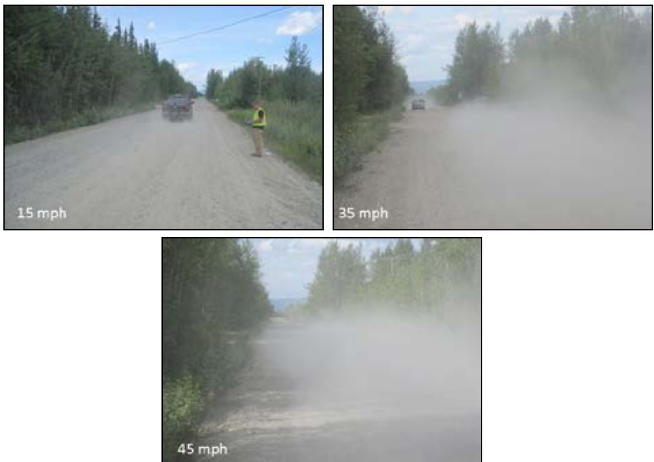
Figure 4.1. Fugitive dust created by a vehicle at different speeds (photos courtesy of Tom Moses)
