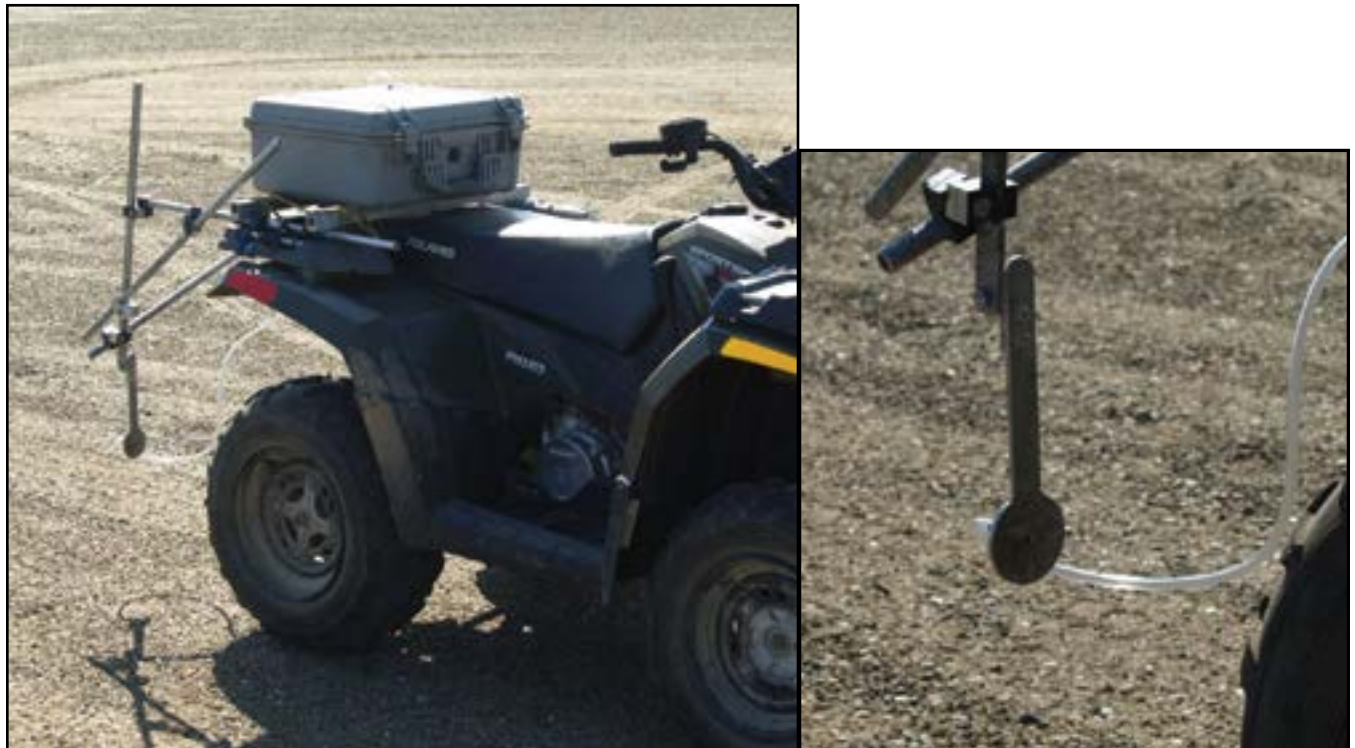
Figure 3.1. University of Alaska Fairbanks DUSTM setup (left) and dust intake detail (right) (from Eckhoff, 2012)
