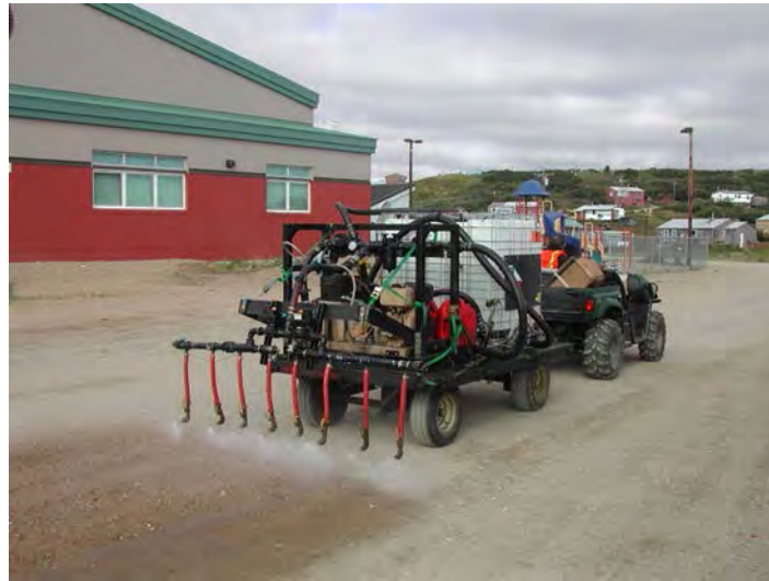
Figure 5.10 Portable applicator developed by the Alaska DOT&PF
