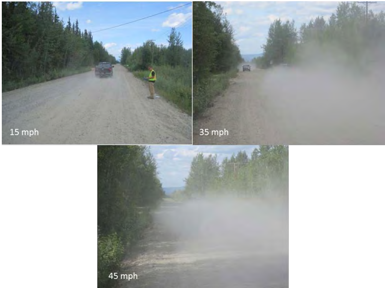
Figure 5.3 Fugitive dust created by a vehicle at different speeds (photo courtesy of Tom Moses)
