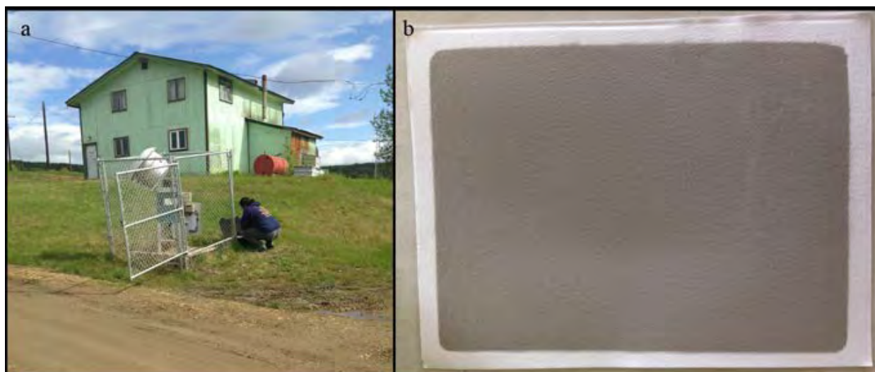
Figure 6. (a) Tribal staff member changing filter at Church site. (b) Filter run for 24-hours with PM 10 deposited on surface.
