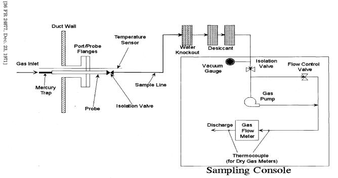
Figure 30B-1. Typical Sorbent Trap Sampling System
