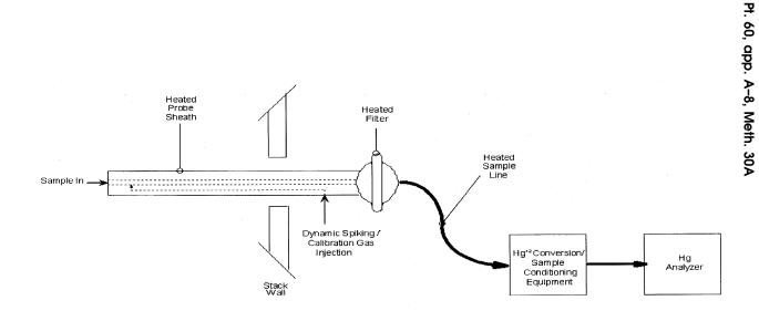
Figure 30A-1: Example Hg Measurement System
