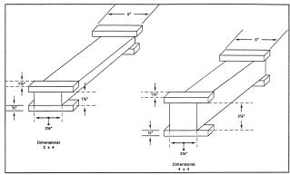
Figure 28-2. Test Fuel Spacer Dimensions.
