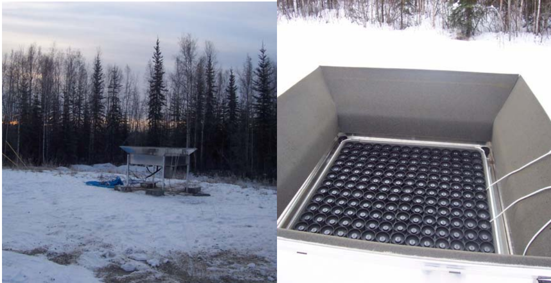
Figure 2.2 Doppler sodar at the NWS site in Fairbanks. (Left) Doppler sodar antenna installed at the NWS site in Fairbanks. (Right) Closer look at the phased array antenna. It comprises of 196 transducers mounted on four panels and surrounded by sound absorbing cuffs to suppress side lobes and to reduce unwanted background noise. The three white heating cables seen on the right are passed along the base of the antenna elements to thaw the snow accumulated from precipitation. (Photos by the author).
