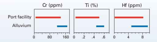
**Figure 4.** Concentration ranges of selected elements in alluvium compared to port facility soil showing significantly higher chromium, hafnium, and titanium in alluvial samples.
