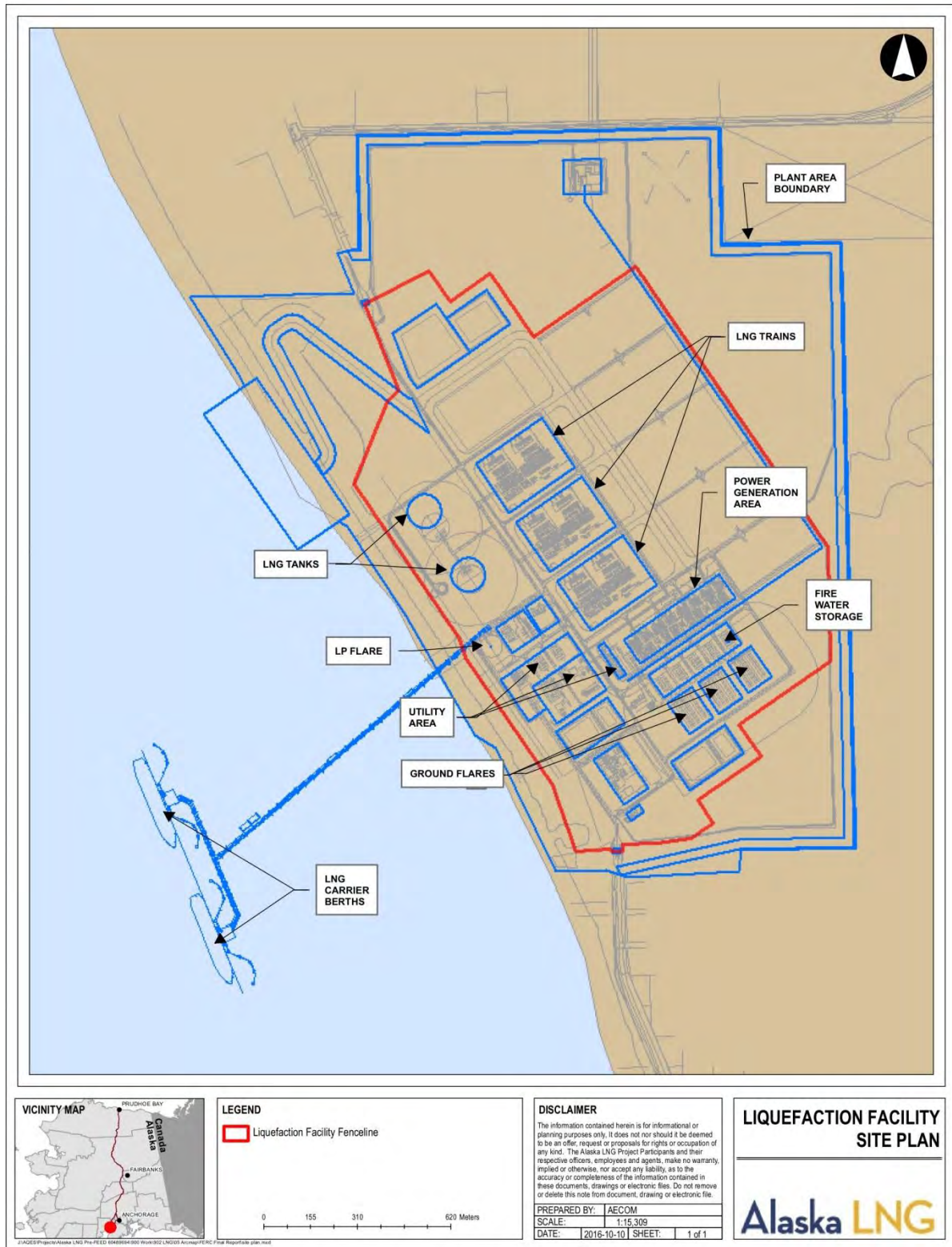
Figure 1-2: Project Proposed Liquefaction Facility Site Plan
