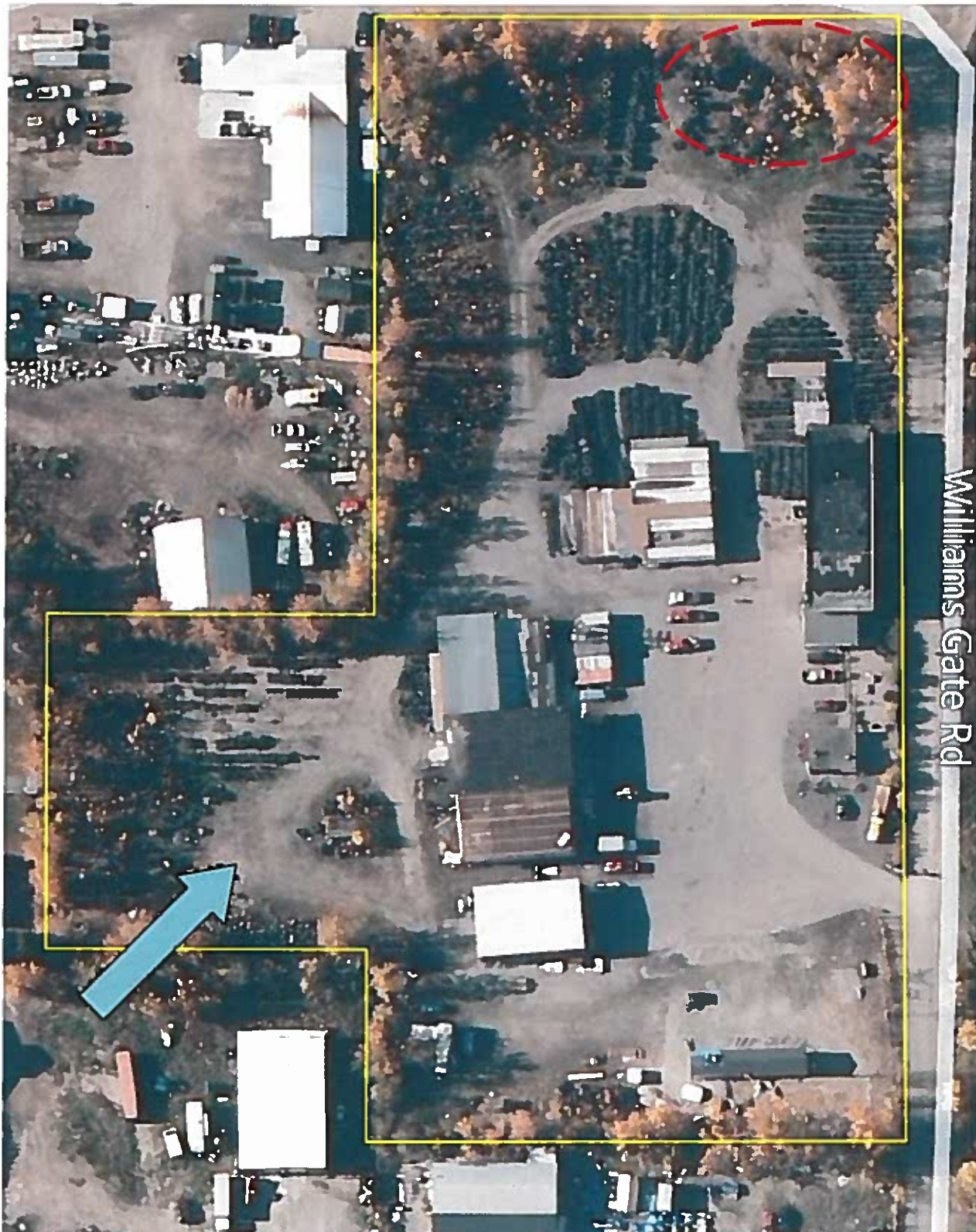
Figure 1. Aerial photo of Giant Tire taken in 2012 (Bing maps). The solid line indicates the approximate property boundary. The dashed circle shows the approximate area of the 1993 soil excavation that included removal of debris. The arrow indicates the regional groundwater flow direction.
