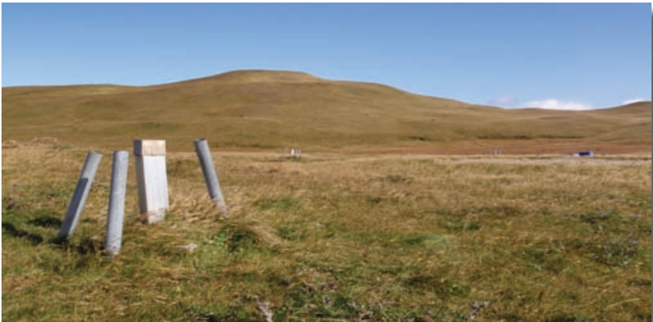
Groundwater monitoring wells
