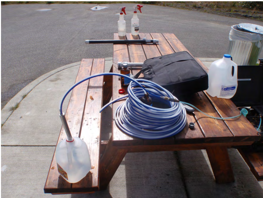
Photo #6: Collecting equipment blank by pumping DI water through decontaminated bladder pump, facing south (8/15/18)
