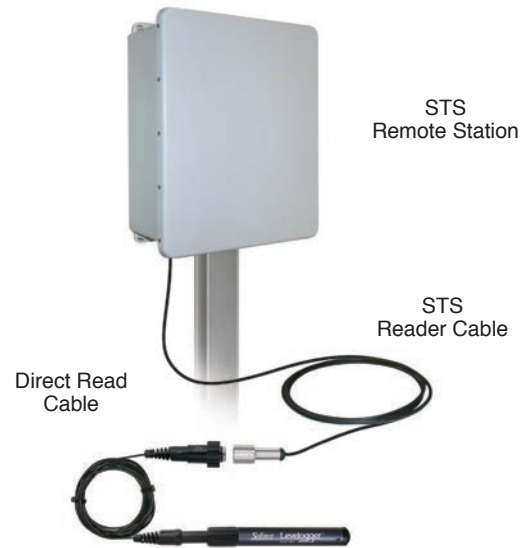
STS Telemetry Systems use GSM/CDMA cellular communication to send remote water level data from Levelloggers to a Home Station PC.
