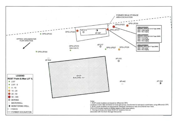
Three temporary monitoring well were installed in November 2009 to reevaluate impacts to groundwater. Water samples were collected from each well and were submitted for laboratory analysis of GRO, DRO, VOCs, and PAHs. None of the sample results from any of the temporary wells exceeded ADEC Table C groundwater cleanup levels (GCLs). A figure showing the well locations and results is presented below:
