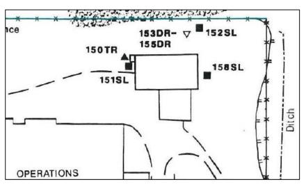
Limited soil removal occurred in late October 1990. A stained area roughly 10 feet wide, 30 feet long, and 6 feet deep was identified and, apparently, removed during this effort. About 14 cubic yards of contaminated soil was removed and disposed of offsite. The removal is not well documented and it is not clear if analytical samples were collected post-excavation. A figure of the excavation is shown below:
