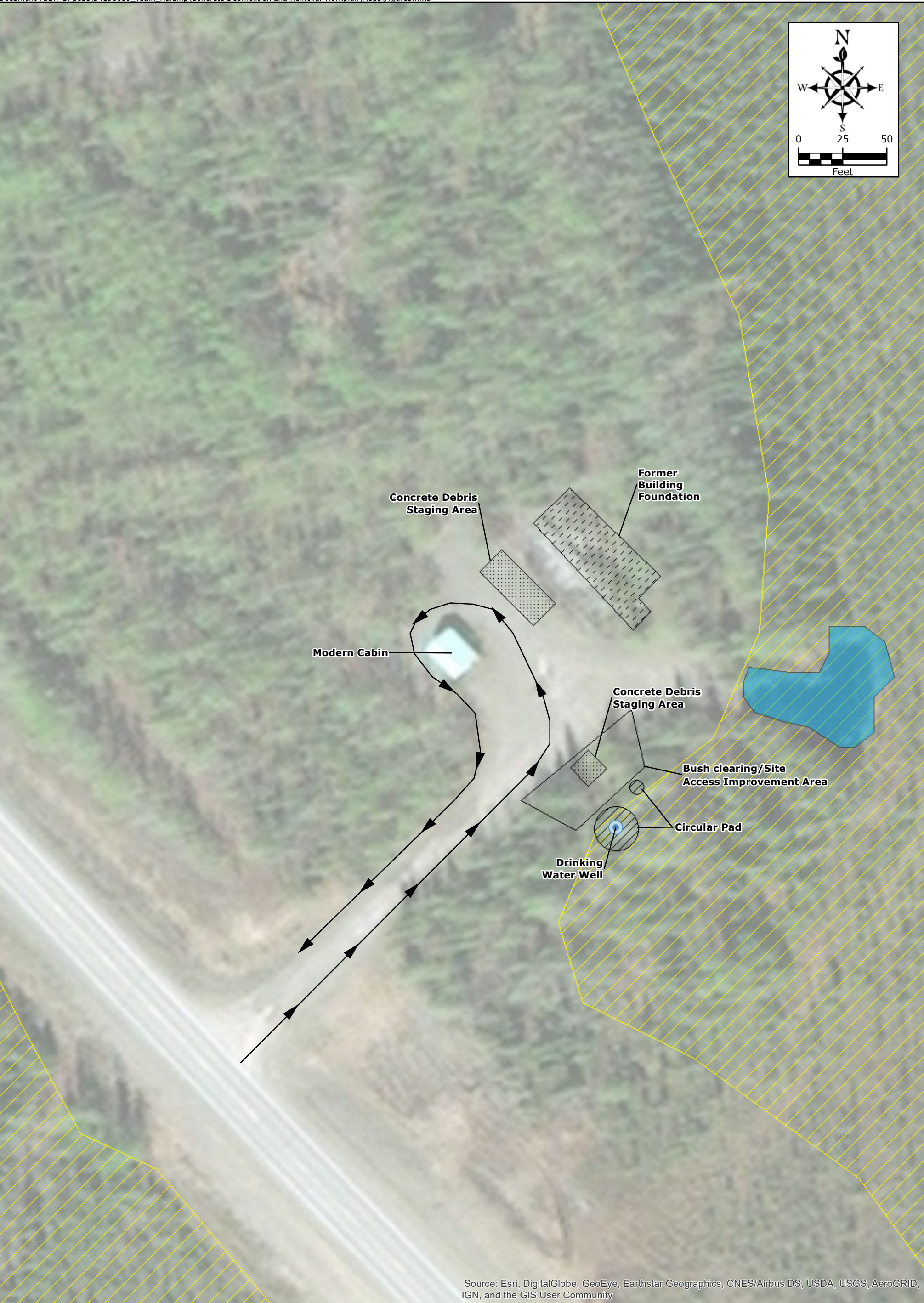
FIGURE 3 TETLIN, NALEMP CANOL PUMP STATION J SITE CONCRETE FOUNDATION REMOVAL MAP
