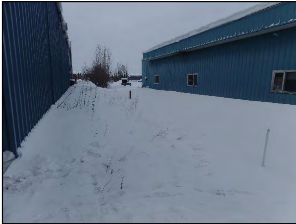
Photo 3: February 13, 2019. Looking south along the west side boundary ditch at MW2 (white stickup) and MW1. MW2 followed by MW1 had higher sums of perfluorooctanesulfonic acid (PFOS) and perfluorooctanoic acid (PFOA) concentrations than MW3 or MW4.
