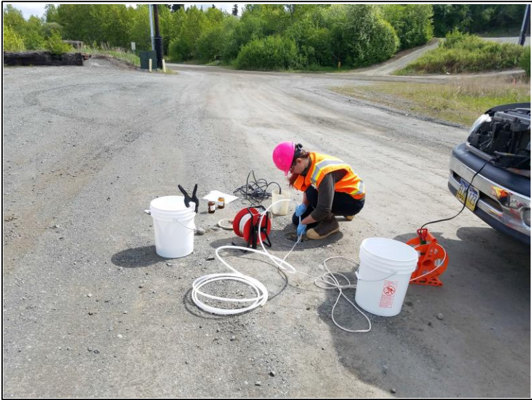
Groundwater sampling at RSE-1. Looking East.
