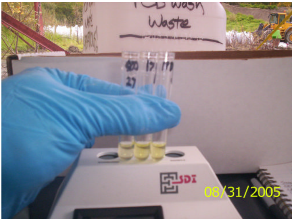
Photo 8. Example of color-dependent concentration. The duplicates “0831-17 (and 17D)-36” have similar color whereas the standard, “STD 27” at 1ppm, is lighter. This shows the duplicate pair to contain less PCB than the 1 ppm standard.
