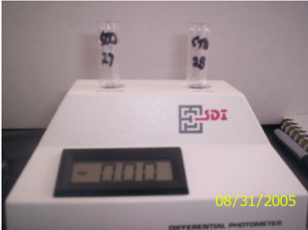
Photo 7. Differential spectrophotometer containing standards for calibration.
