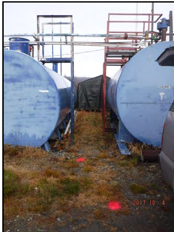
Photograph 6: Proposed test boring locations 1 and 2 (1 is furthest south) identified for collecting Torkelson soil samples.
