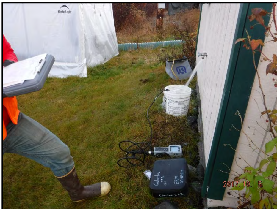
Photograph 10: Eureka Lodge's current drinking water well sample location from outside of well house. Photograph 11 shows the green hose connected this spout to the drinking water well.
