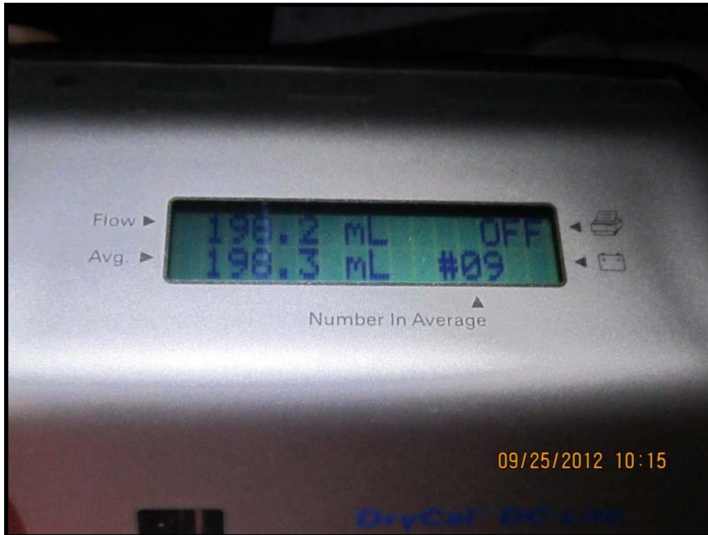
Photo 11: TA-01 air sample collection flow rate.
