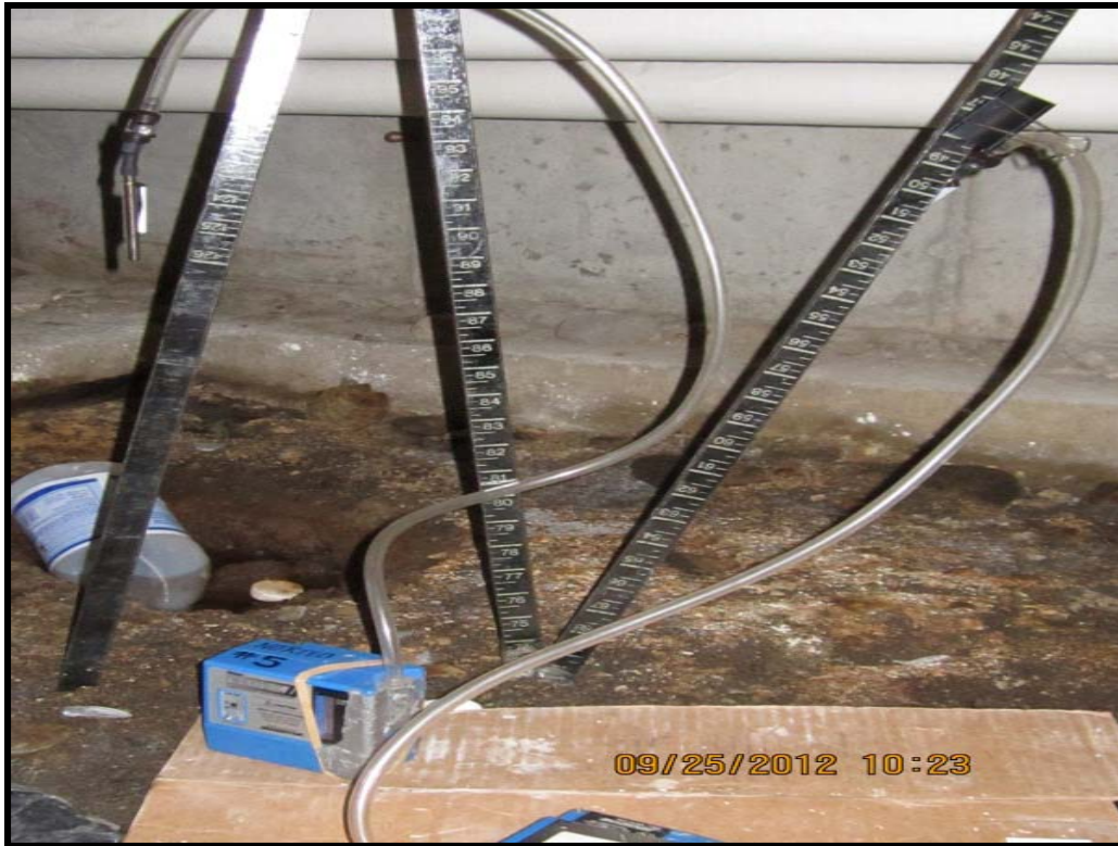
Photo 13: Air sample collection setup. TA-01 on left and TA-02 on right.
