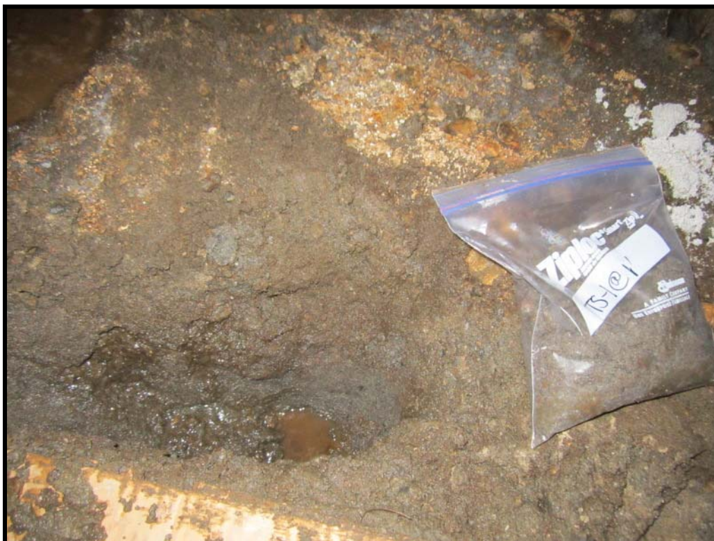
Photo 2: TS-1 soil boring. Showing soil types and groundwater encountered.
