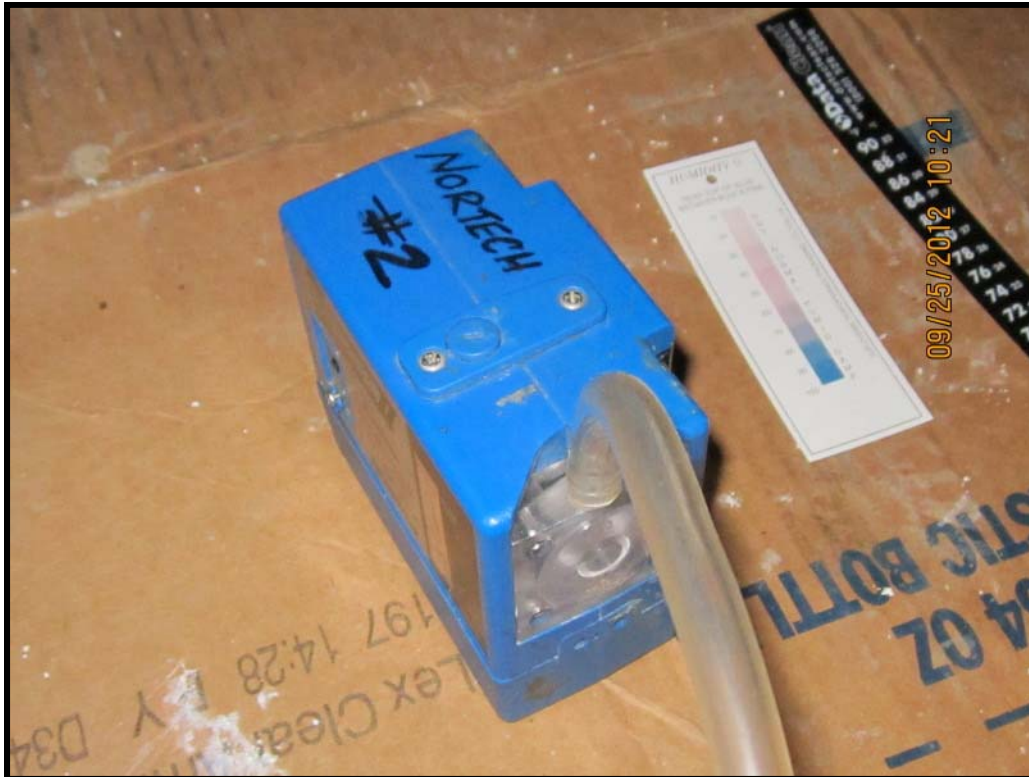
Photo 9: Pump used for collection of TA-02.
