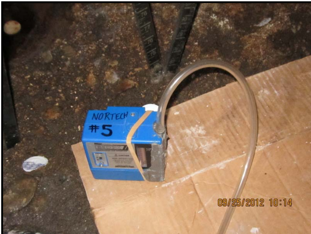
Photo 8: Pump used for collection of TA-01.
