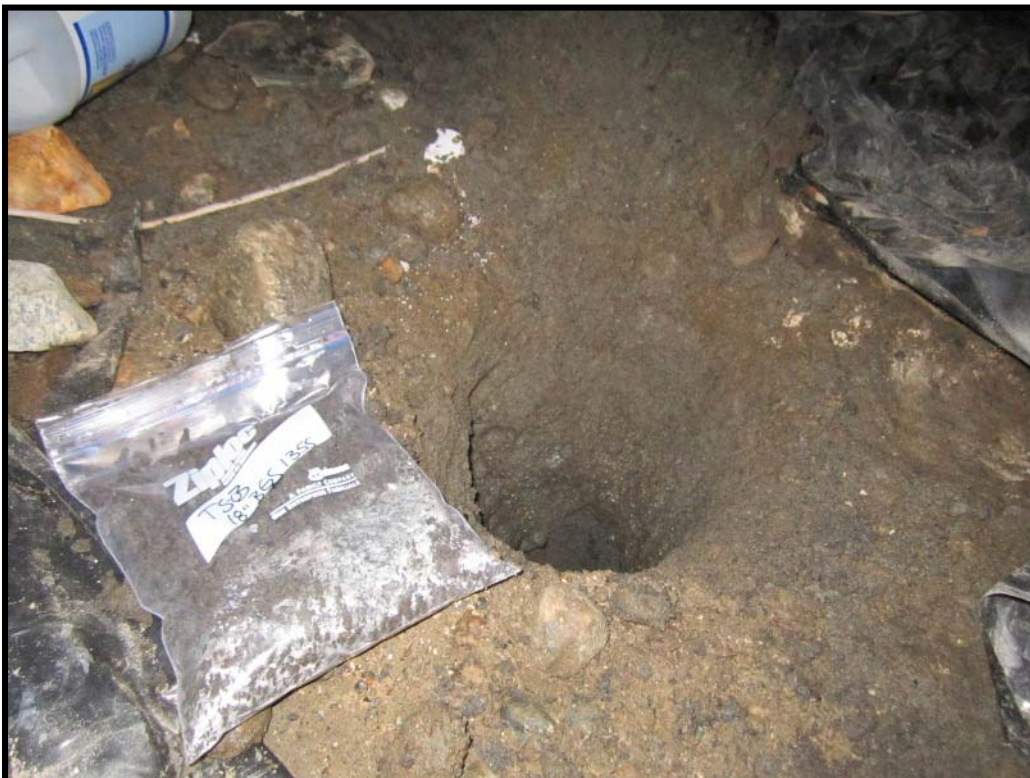
Photo 4: TS-3 soil boring location. Soil types and capillary fringe encountered.
