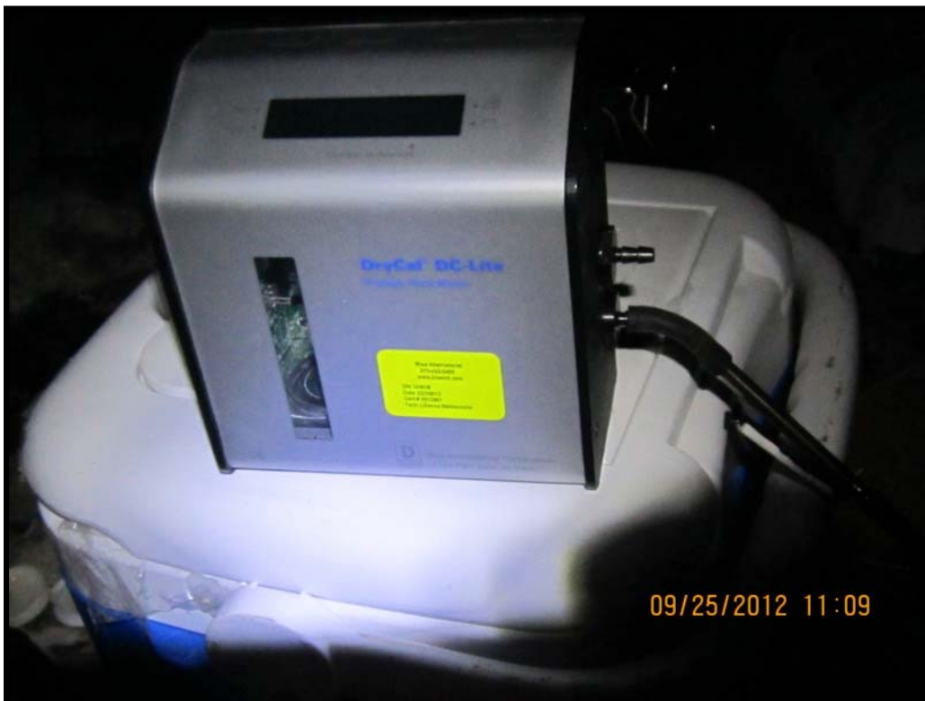
Photo 10: DryCal calibrator used with calibration tube to control air sample collection flow rates.
