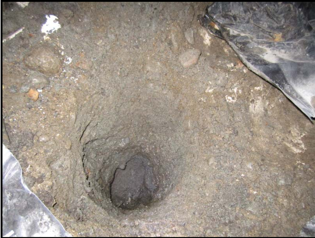
Photo 5: TS-3 soil boring showing capillary fringe.
