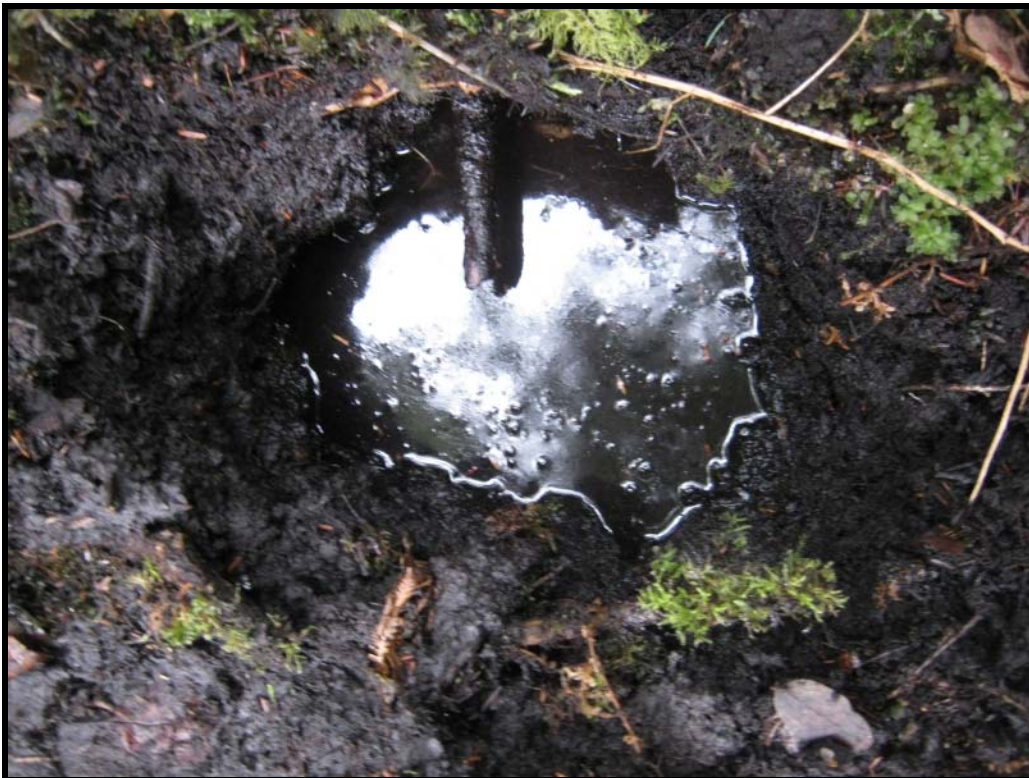
Photo 2: TP2 with groundwater at 4' below ground surface
