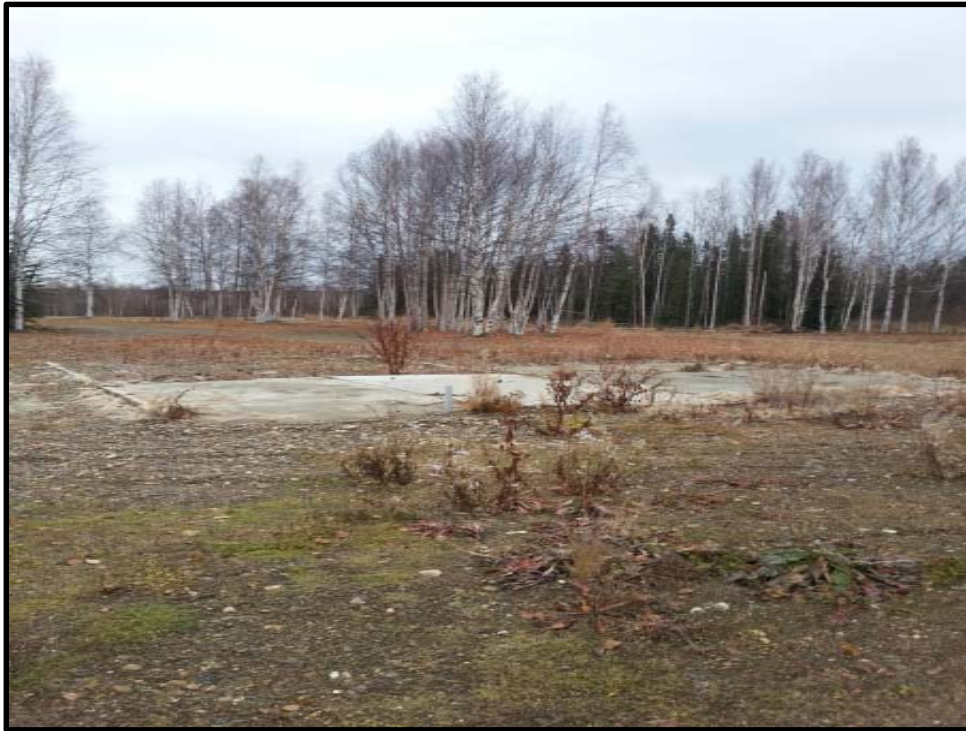
Photo 1: LIDAR Garage slab, photo taken facing southeast. Collected composite samples for PCBs near the former backdoor (typical of other suspect area samples at this location)
