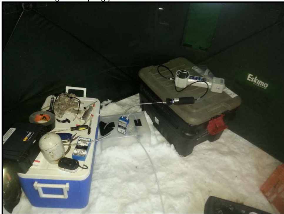
Photo 6: Soil gas sampling apparatus in use inside a heated portable ice fishing tent during the helium leak-test on the sampling train prior to sampling.
