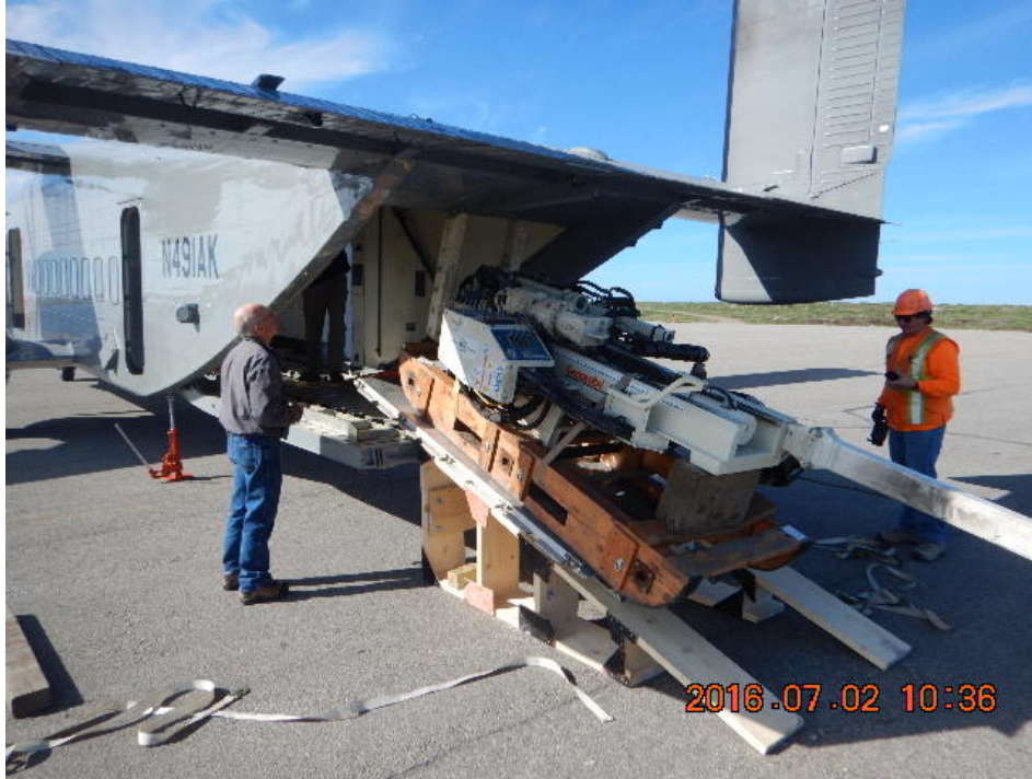
Photograph 17: Loading the drill rig mast onto the Sherpa for transport. Facing west.
