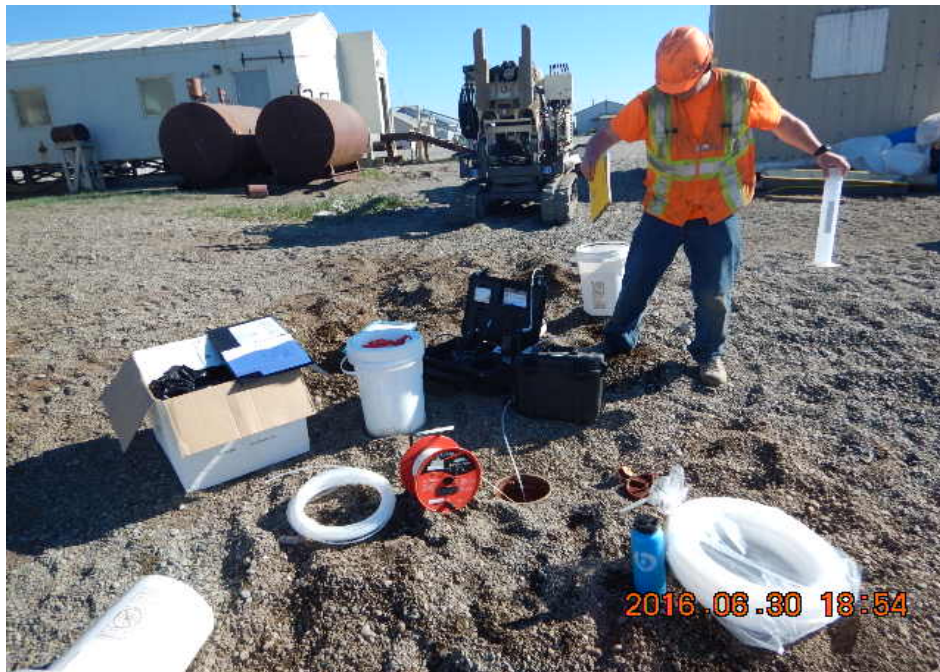
Photograph 2: Setting up at 16GAMMW03 for well development. Facing south.
