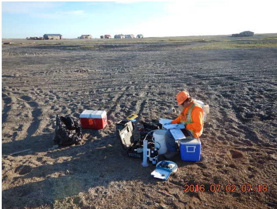
Photograph 14: Purging well 16GAMMW04 for sampling. Facing north.
