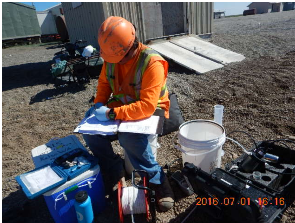
Photograph 10: Purging well 16GAMMW01 for sampling. Facing southeast.
