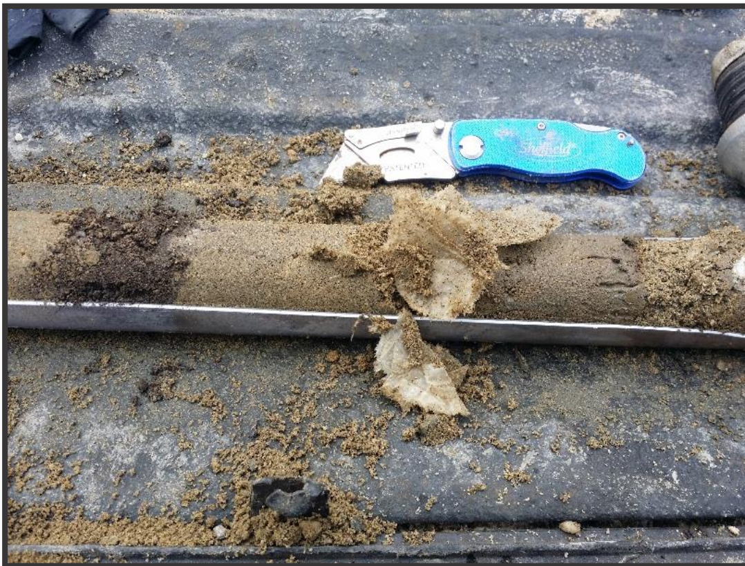
Photo 4: A closer look at the poly sheeting. Also, note the black sands encountered at several of the boreholes. These sands were typically found at about three feet bgs.
