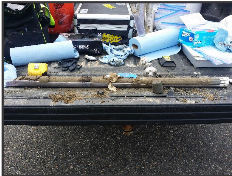
Photo 2: Borehole BH-02 sample from two to six feet. Note polyethylene sheeting in center of sample sleeve.
