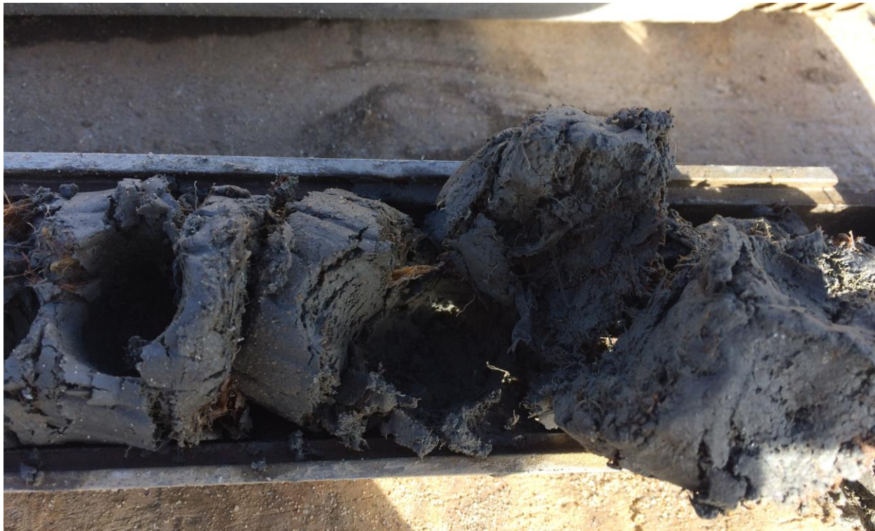
Core from C6 at 5 feet bgs with high amounts of organics in silt.
