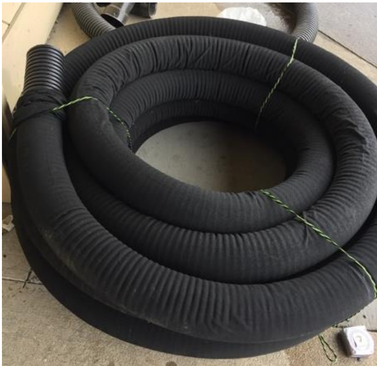
Sleeved piping used for SVE collection
