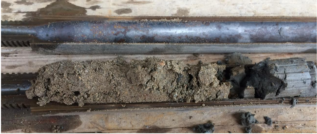
Split spoon sampler with core from C4. Transition to silt beginning at 4.75 feet bgs.
