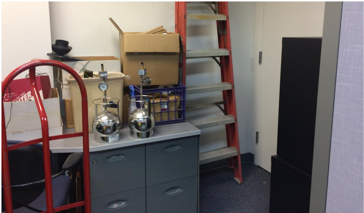
Indoor air sampling in Suite 595 with duplicate. Location is where former dry-cleaning machine was
