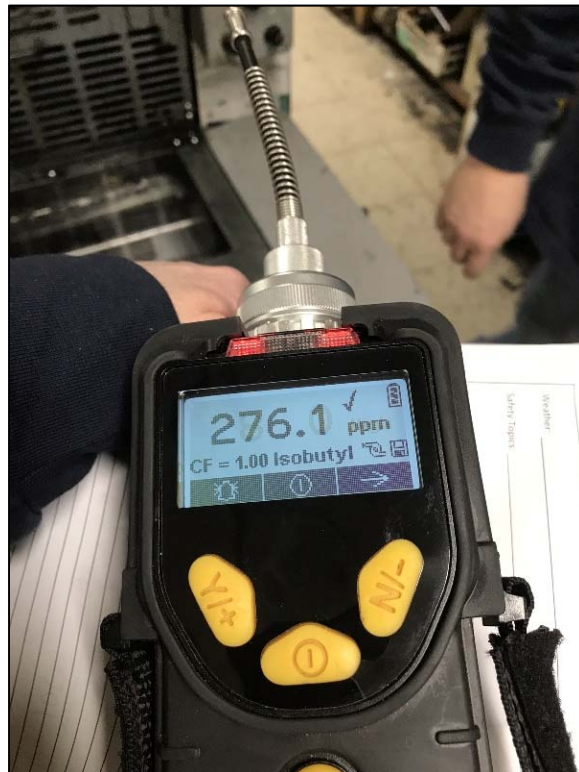
Photo 2: Typical indoor air reading near a printing unit during indoor air quality assessment.
