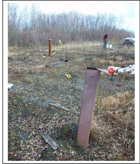
Photo 2: Looking north, monitoring wells RA-MW-4 (near) and RA-MW-3 (distant) are typical stick-up wells. (5/18/2010)
