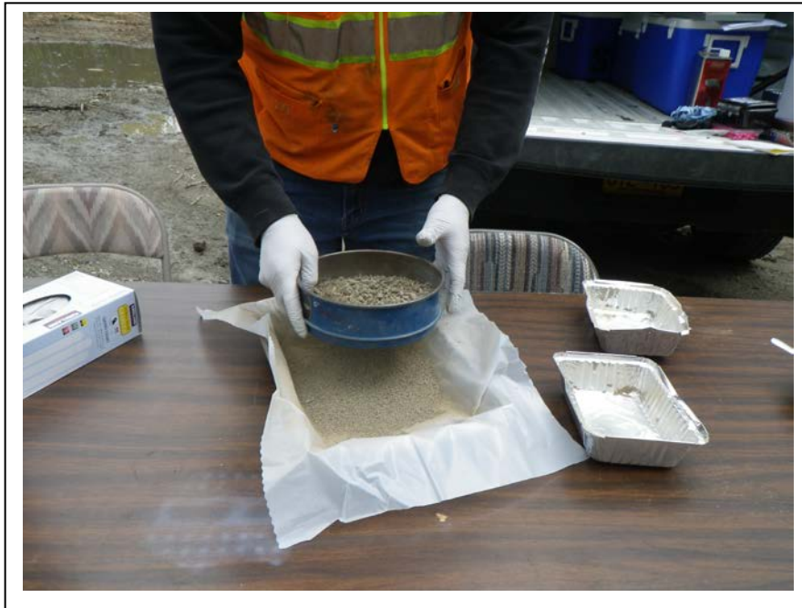
Photo 4: Hand sieving sub-portion through a #10 (2mm) sieve.
