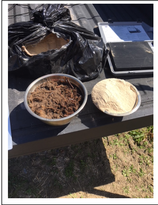
Photo 7: Bench scale impact area sample (left) and phosphate (right).
