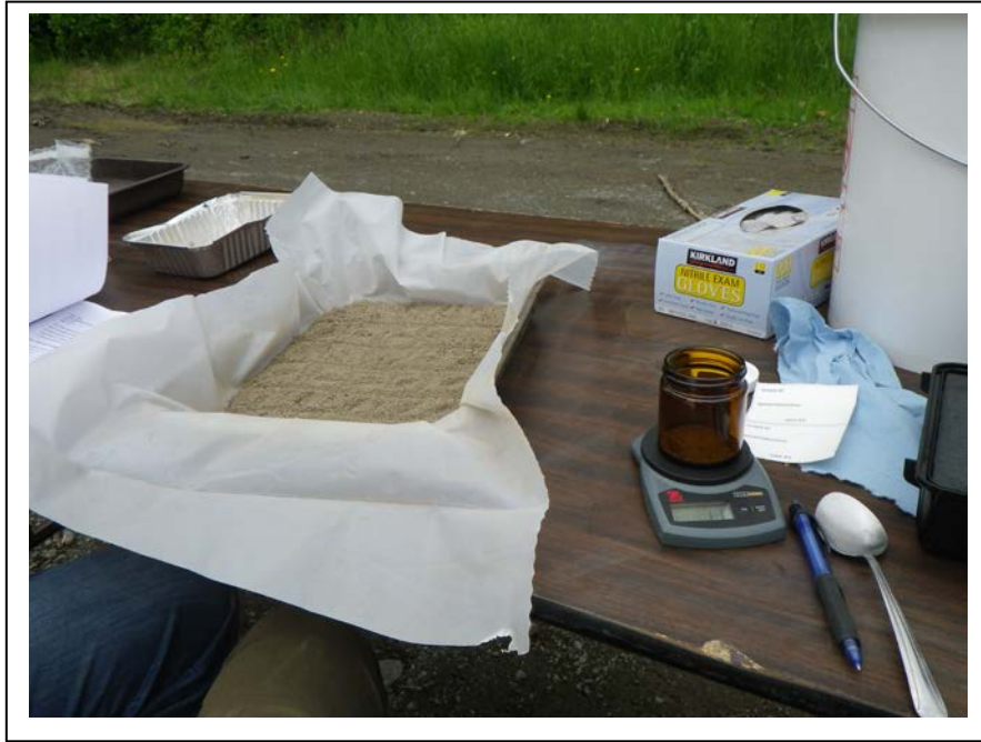
Photo 5: Preparing to collect a 1 mg sample for lab analysis.
