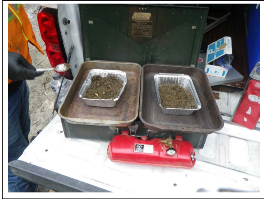
Photo 3: Drying the sub-portion sampling prior to sieving.
