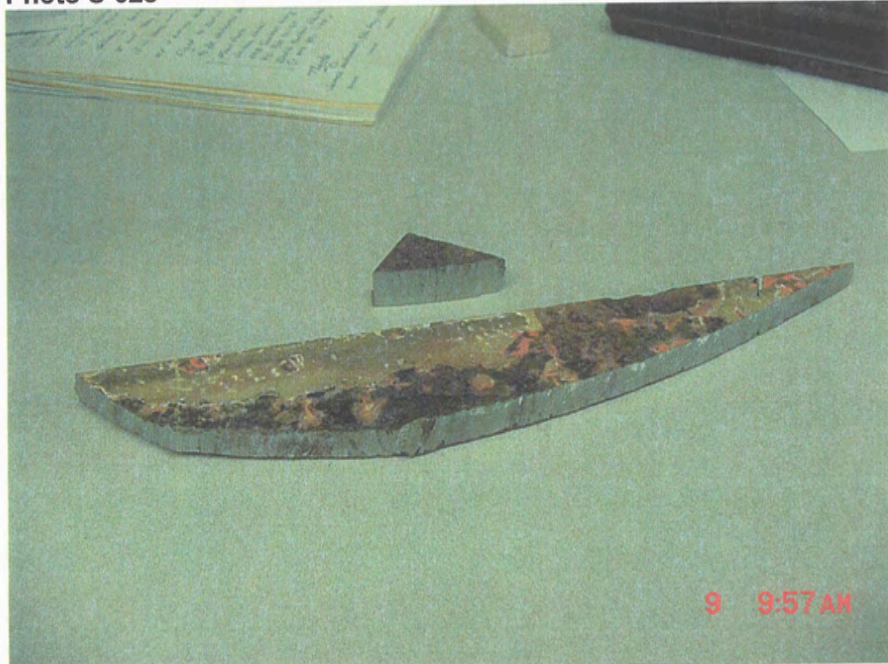
Grid 7/C – Curved sample removed from beam, bottom flange, June 2003
