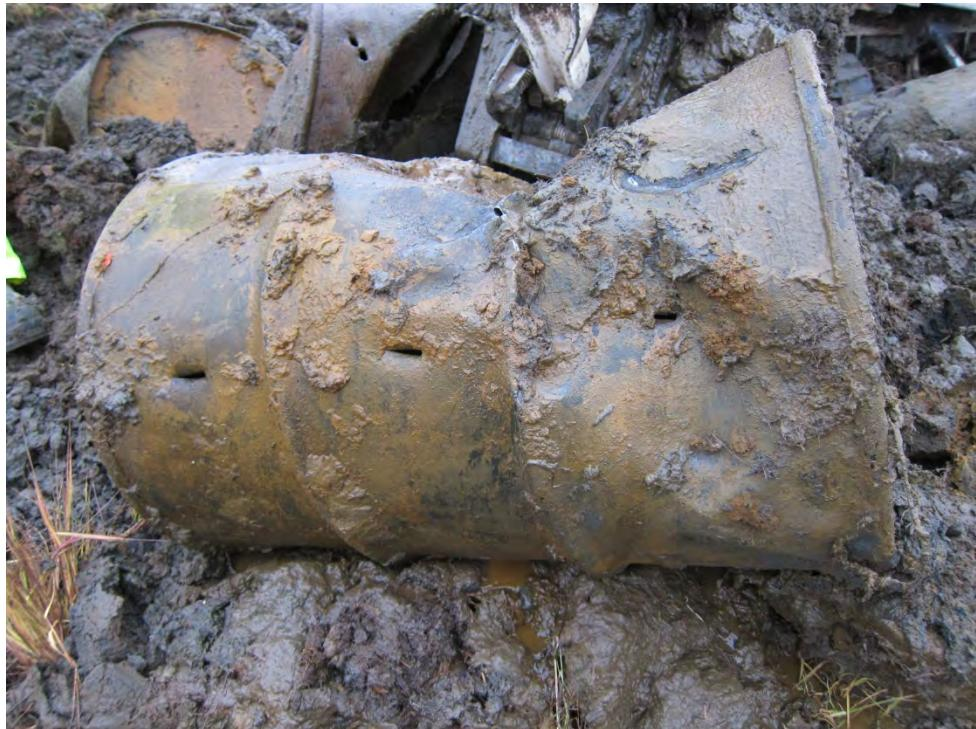
**PHOTOGRAPH 6: DRUMS APPEAR TO HAVE BEEN PUNCTURED PRIOR TO BURIAL.
