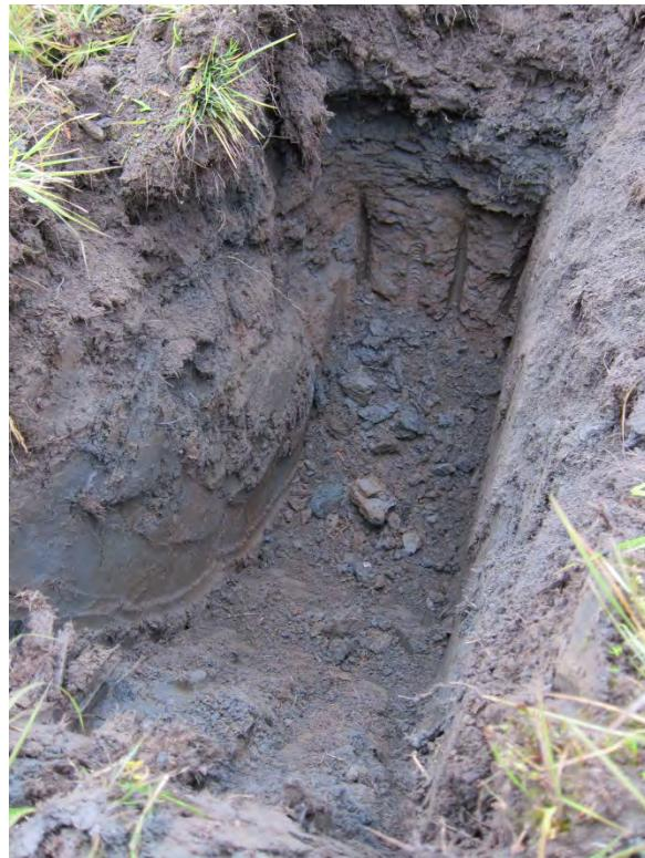
**PHOTOGRAPH 12: TEST PITS EXCAVATED TO APPROXIMATELY 5' BELOW GROUND SURFACE. SOIL HORIZONS TYPICALLY CONSIST OF 0-1' ORGANICS AND 1-5' SILT WITH SOME NATIVE WOODY MATERIAL. 10/05/2013.**
