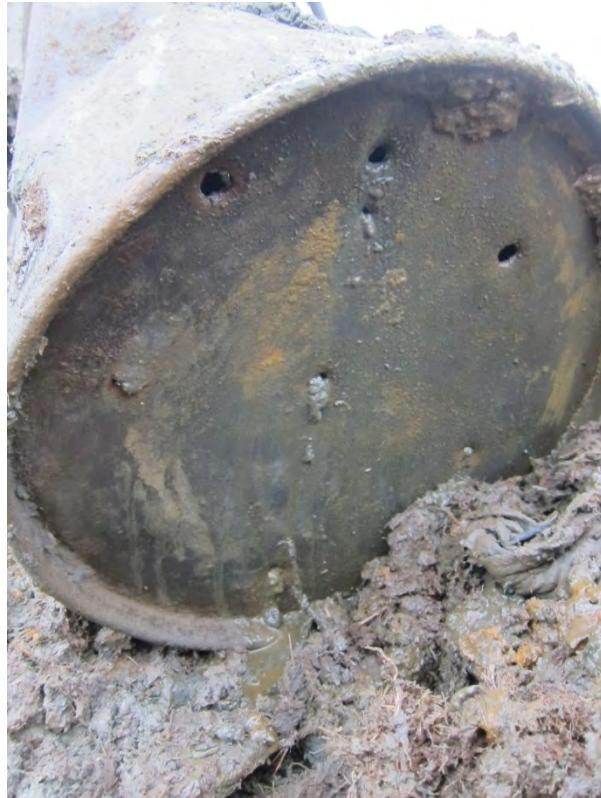
**PHOTOGRAPH 7: DRUMS APPEAR TO HAVE BEEN PUNCTURED PRIOR TO BURIAL.**
