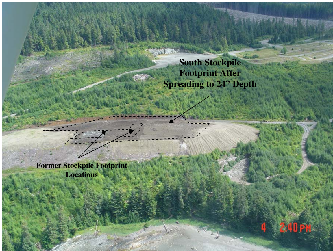
Photo 4. Configuration of South Stockpile Following Spreading.
