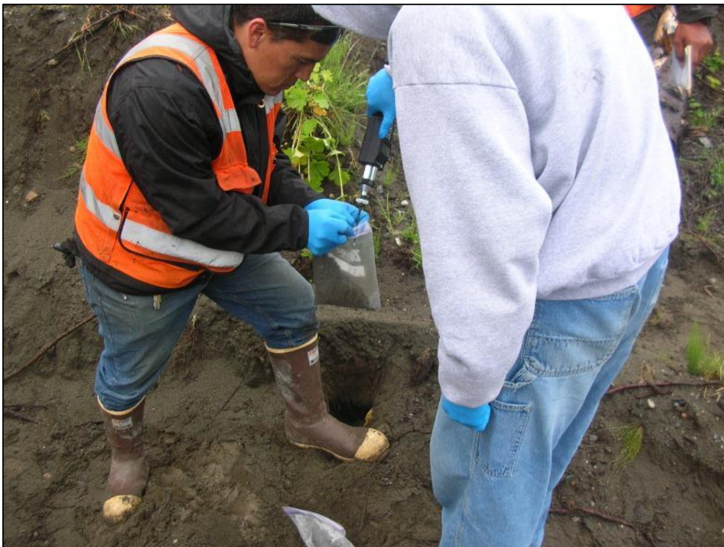
Photograph 2. Crew conducting field screening using PID.
