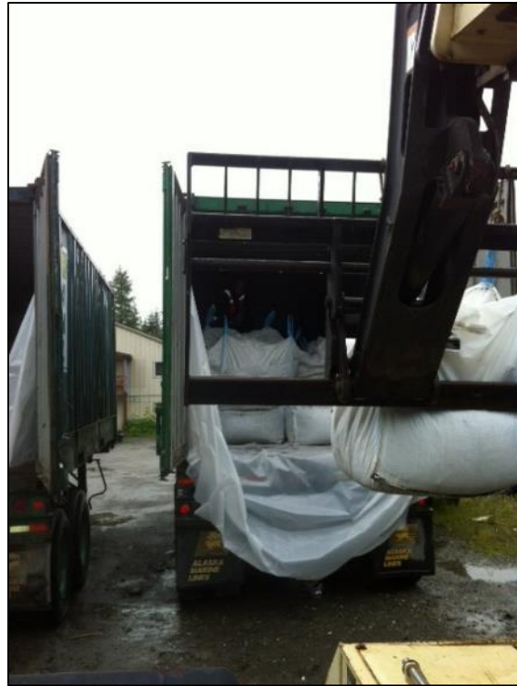
Photograph 1. Loading PCS filled Super Sacks® in shipping container.
