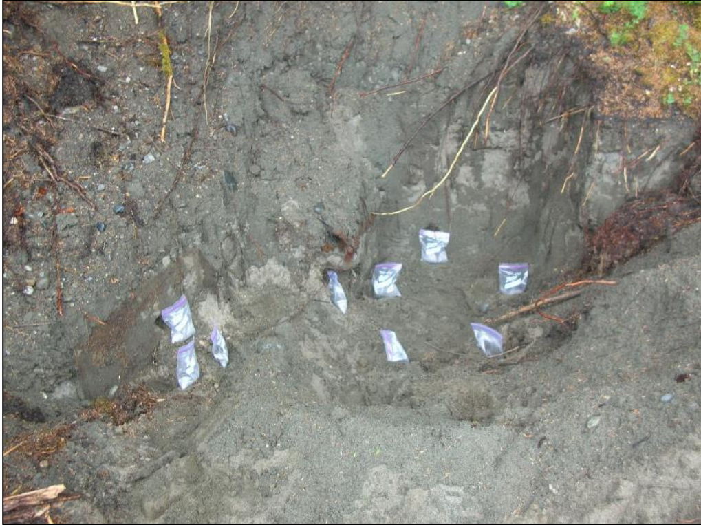
Photograph 7. Drain Area excavation showing screening samples.
