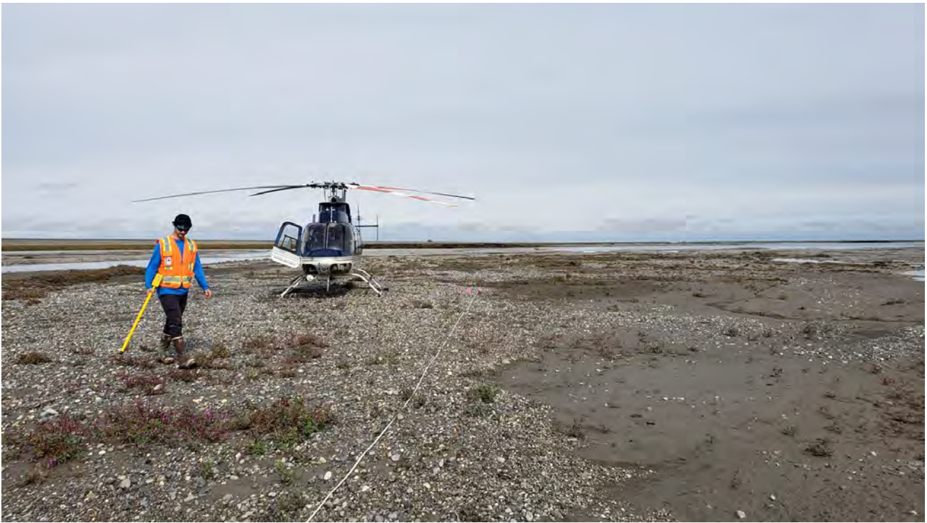
Photo 3: SLR staff conducting site screening for large magnetic anomalies on typical gravel bar ground surface using a magnetometer. Photograph faces north.
