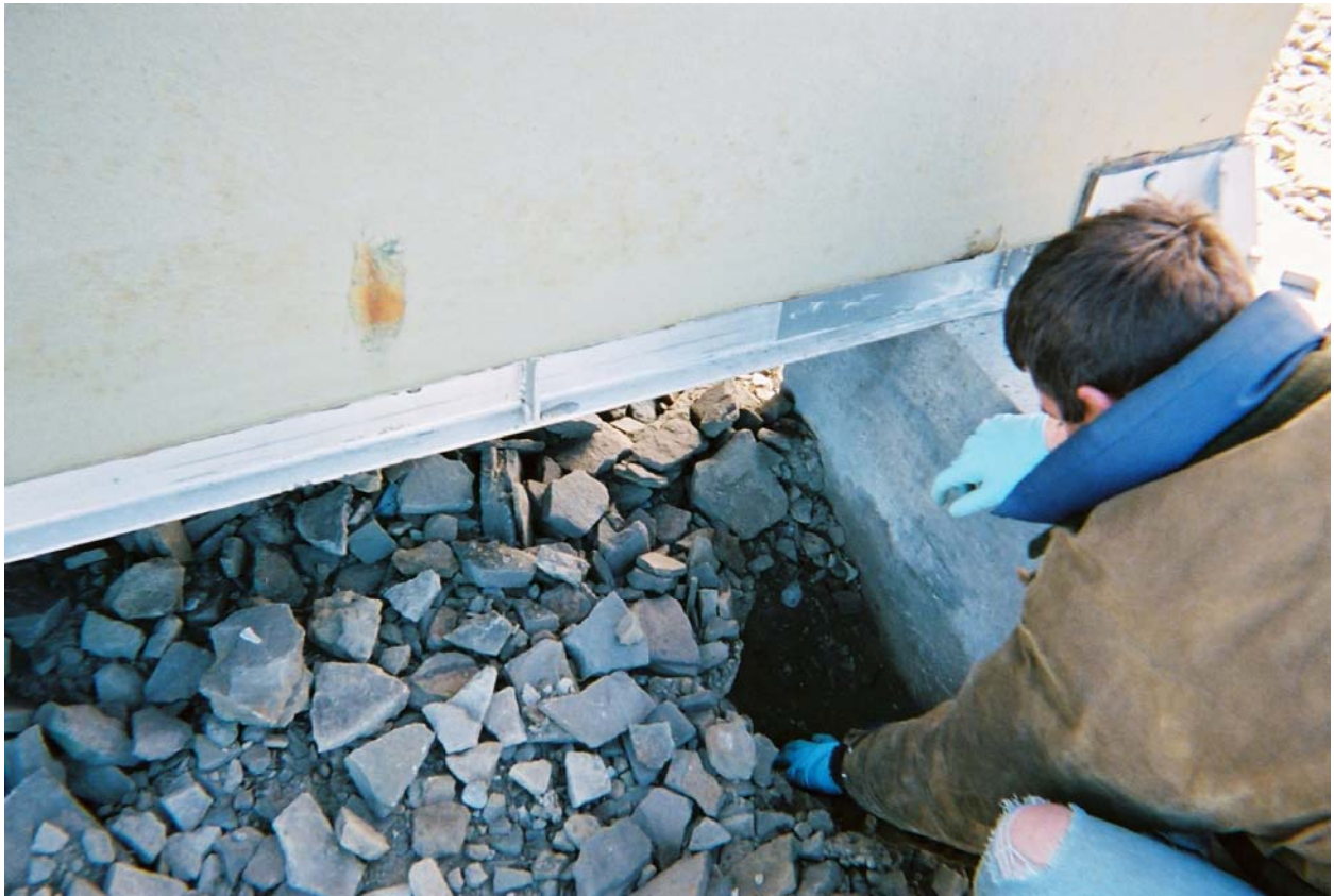
Collecting PID samples around the perimeter of the Generator Module.
