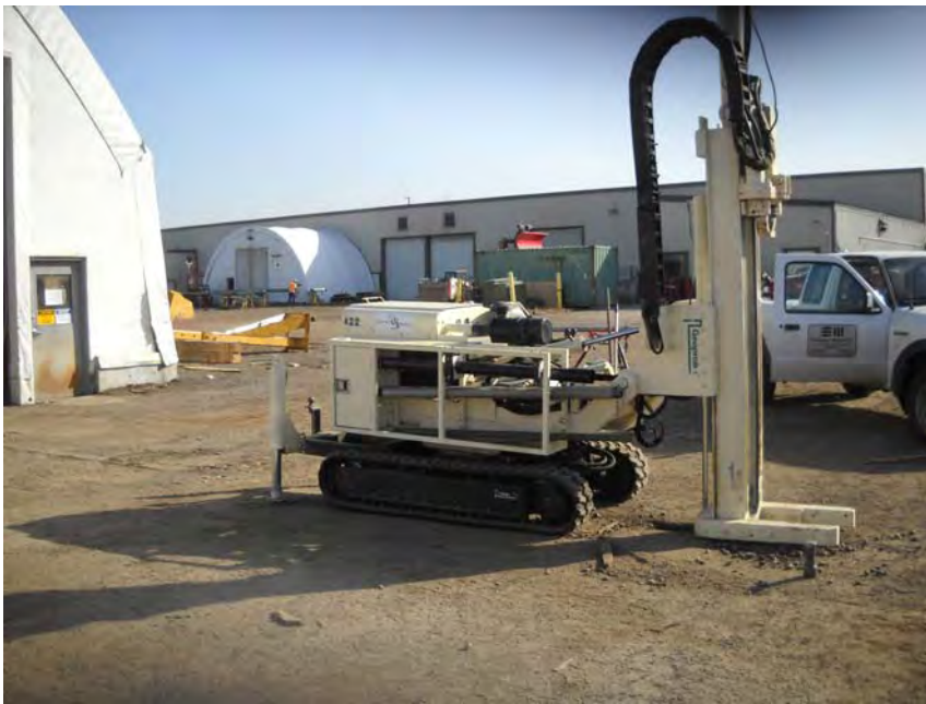
Photograph 7: Looking northeast, Boring B2 was advanced in the southwestern portion of the property, near October 2010 Sample SS3. (April 2011)
